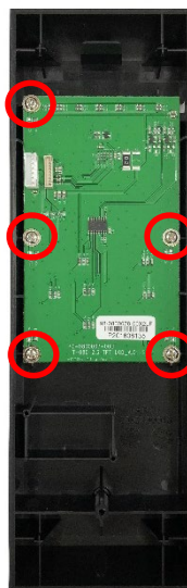
ML240P Series LCD panel with five screws
