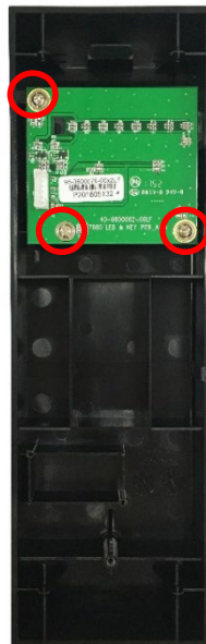
ML240/MA2400C Series LED panel with three screws
