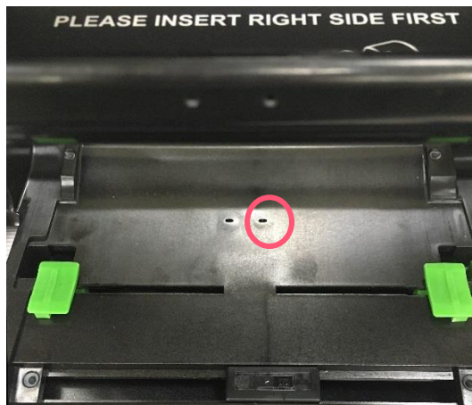
Gap sensor (receiver) (Fixed position, shift 4 mm to right)
