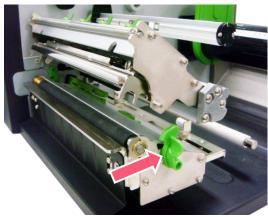
**1.** Lift the handle to open the printer right side cover. Push the print head release lever to open the print head mechanism.
