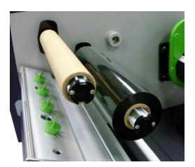
2. Install the ribbon and paper core onto the ribbon supply spindle and ribbon rewind spindle. Make sure the ribbon & paper core are set at the center of the spindle. (User can refer to the ruler on the spindles.)
