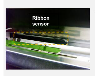
3. Thread the ribbon through the ribbon sensor slot and then through the open space in between print head and platen roller.
