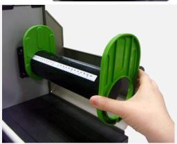
**2.** Remove one label roll guard from the label spindle.
