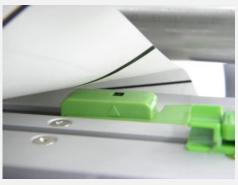
**6.** The media sensor position is moveable. Please make sure the gap or black mark is at the location where media gap/black mark will pass through for sensing.
