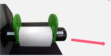
4. Place media roll on label supply spindle. Replace label roll guard. Make sure the label roll guard position of each sides are the same as the length of the label. Please check the outside edge scales are both close to the label width.
