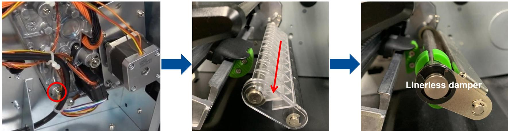
10. Plug the tear (or cutter) module mini DIN cable connector into the printer receptacle.
