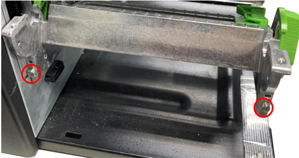
5. Move the label guide (green) to the outermost side to install the rubber cover and stick the linerless pad on the lower base.
