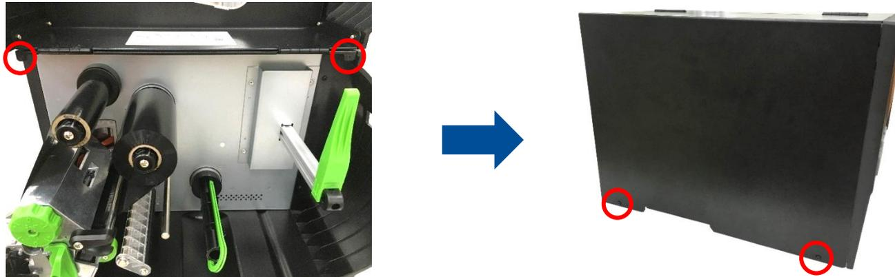
4. From the back of the printer lift up and tilt the top of the side cover up until the tabs along the lower edge disengage from the slots in the printer base frame and remove the side cover.
