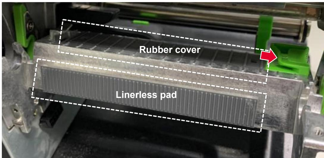
6. Install the linerless roller.
