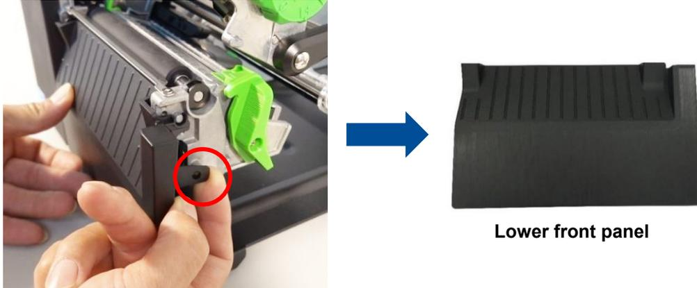
4. Reassemble the parts in the reverse procedures.
