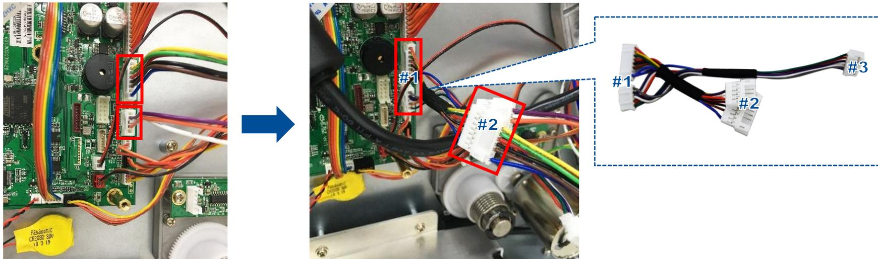
5. Fasten the two screws (fastened by  $5.5 \text{ kg} \pm 15\% \text{ kg-cm}$ ) on the GPIO mounting plate first. Then, aligning the GPIO board to the two locating holes on GPIO mounting plate and fasten another two screws (fastened by  $5.5 \text{ kg} \pm 15\% \text{ kg-cm}$ ) to secure the GPIO board. Insert the rest connector of GPIO transfer cable (#3) to GPIO board. Fasten the two screws and the two hexagon screws on the GPIO interface board on the rear of printer.
