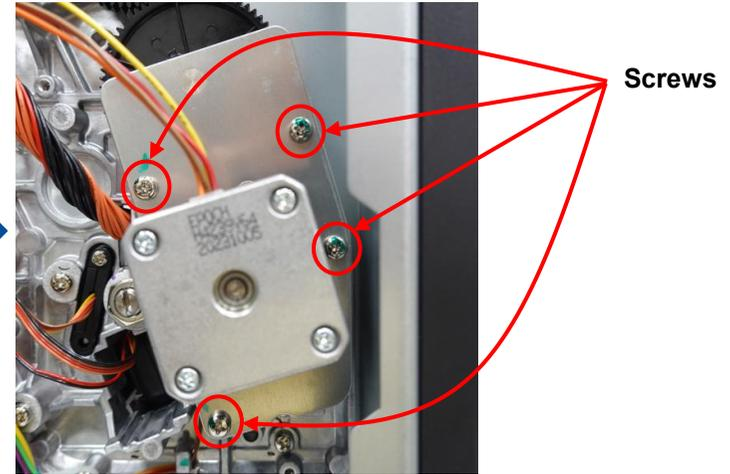
4. Remove/Replace the stepping motor assembly. (including gears and stepping motor)
