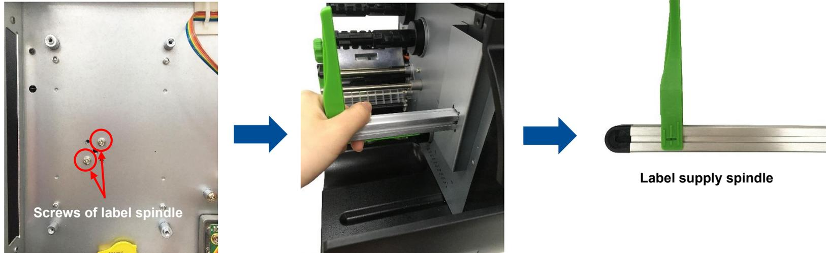
5. Reassemble the parts in the reverse procedures.
