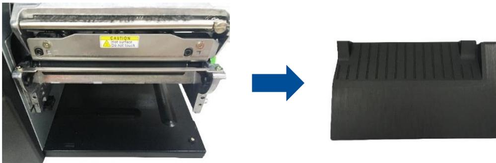
3. Open the cutter module panel. Install cutter module cable on printer cable socket as indicated.
