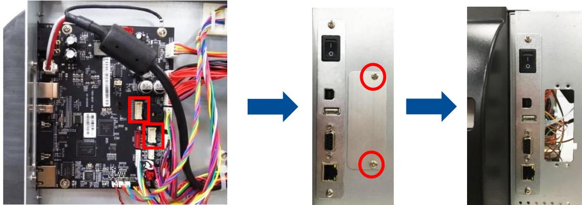
4. Install the slot-in wireless housing on the rear of the printer and fix the two screws. ( $5.5 \text{ kg} \pm 15\% \text{ kg-cm}$ ) Connect another side of the cables to the slot-in wireless transfer module housing board. Reassemble the parts in the reverse procedures.
