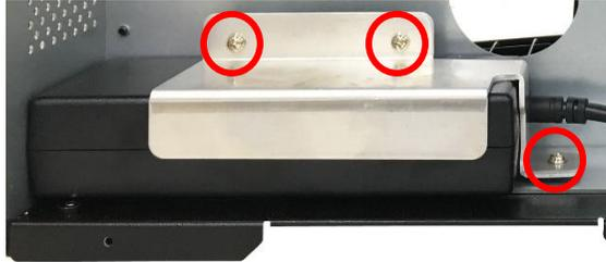
4. Remove one screw (fastened by  $7.5 \text{ kg} \pm 15\% \text{ kg-cm}$ ) and disconnect one connector on main board. Loosen three cable ties to remove/replace the power supply unit.
