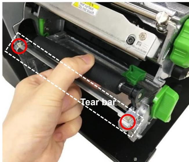
4. Fasten the two turning screws (M3\*4L; provided in the kit/ fastened by 7.5 kg±15% kg-cm) on printer mechanism as indicated.
