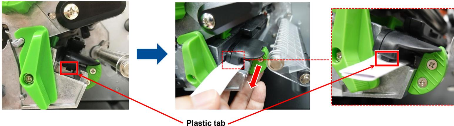
5. Remove/Replace the gap/black mark sensor.
