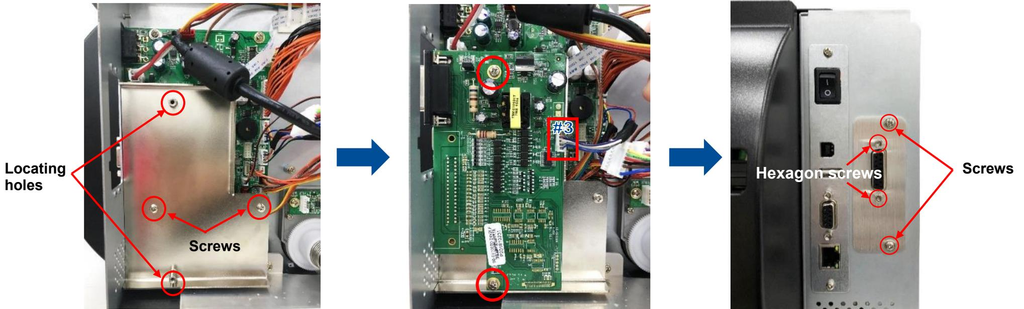
6. Reassemble the parts in the reverse procedures.
