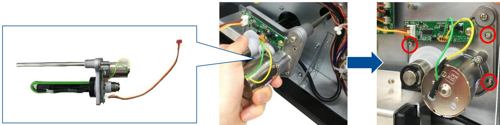
5. Connect the rewinder module cable to the main board socket (CON26/ red).
