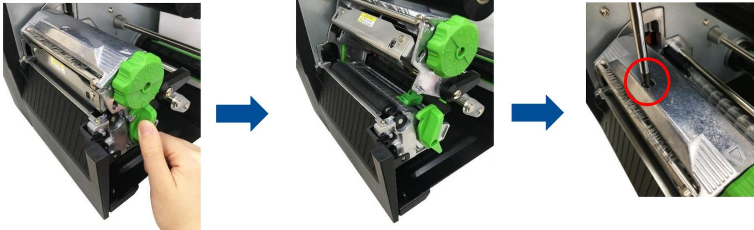
5. Disconnect the printhead harness to remove/replace the new printhead assembly.
