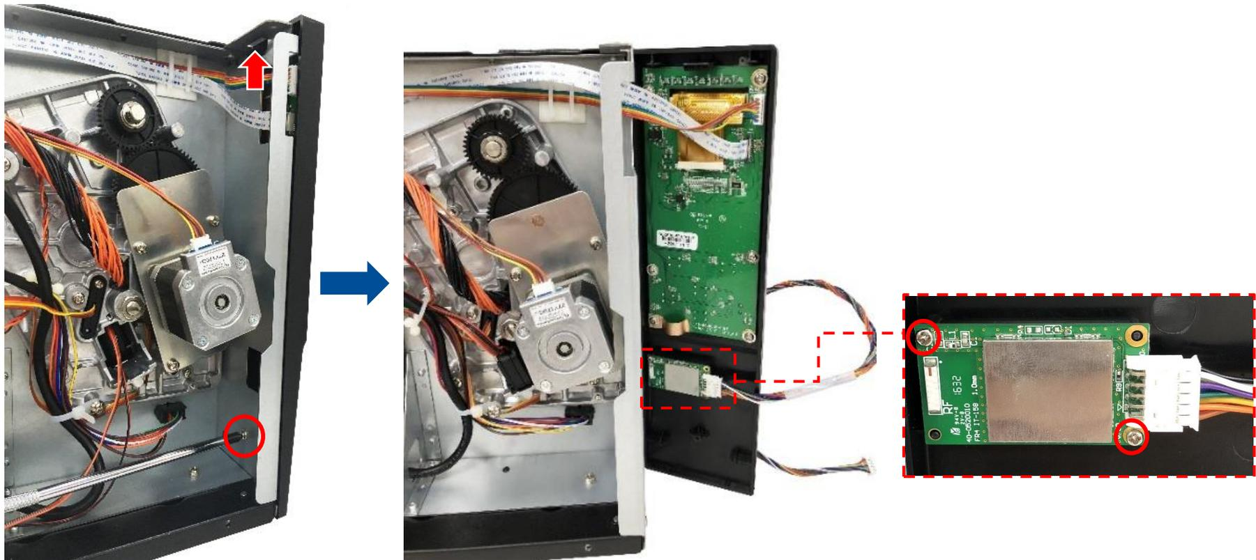
4. Connect the Bluetooth module cable on the main board (CON13) as indicated.
