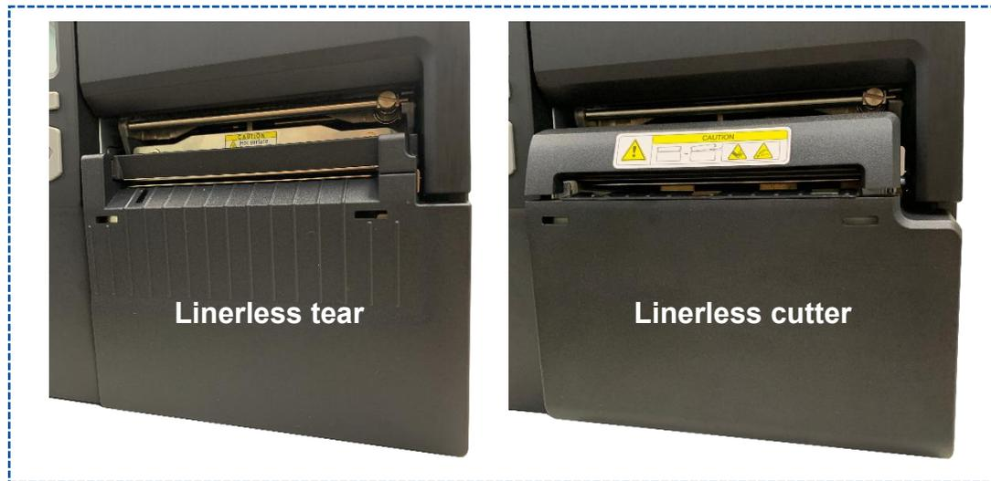
12. For the linerless cutter module, the cutter tray is mounted on the cutter panel as required.
