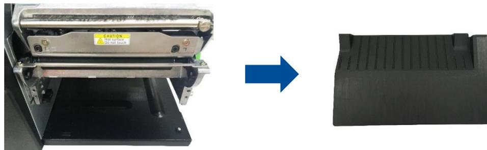
3. Install peel-off sensor module cable on printer connector as indicated.
