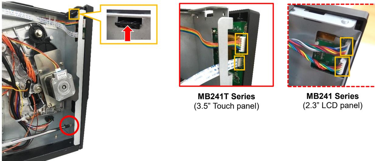
4. Remove/Replace the control panel assembly.
